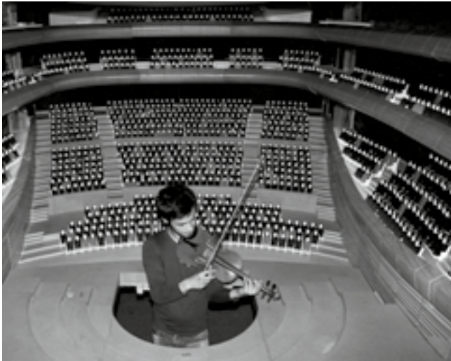
NAGATA BUILT A 1:10 SCALED MODEL FOR HIS ACOUSTIC-TESTS
